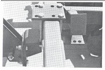
3a. Bracket #2 is a modified short universal disk bracket (PN 8H1546) that mounts to the disk main frame as shown above. Secure using a 1/2 x 5 x 6-1/8" mounting plate (PN 8H1340) and four 5/8 x 8" bolts.
